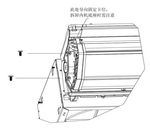
1. remove the screws fixed to the evaporator to the air duct assembly.
