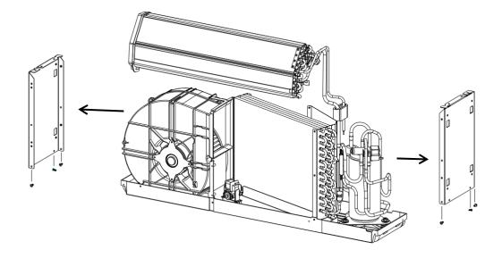
VIII. Dismantling of exhaust duct assemblies
