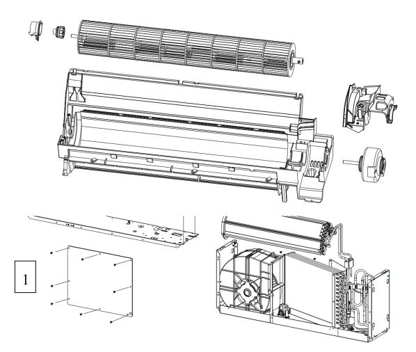
4. remove the screws attached to the base and the side plates and remove the side plates.
