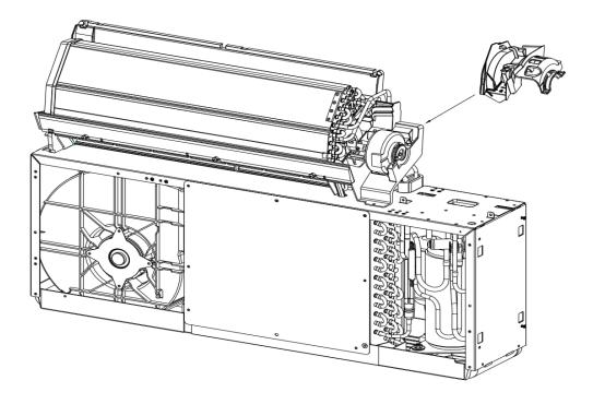
1. remove the screws fixed to the evaporator to the air duct assembly.
