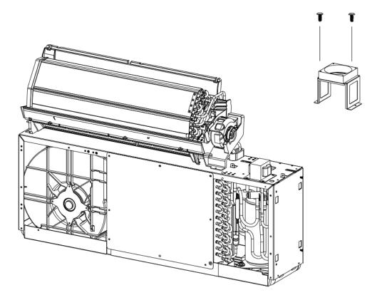
4. remove the screws that fix the reactor and remove the reactor.
