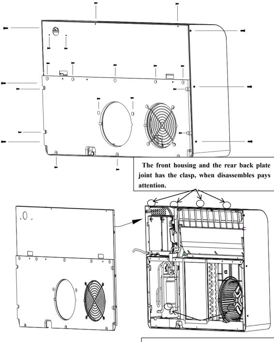
The front housing and the rear back plate joint has the clasp, when disassembles pays attention.
