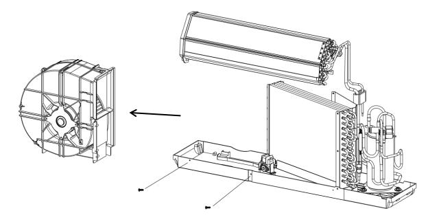
2. remove the 4 screws on the outside of the volute, loosen the nut fixed on the motor shaft, remove the nut, pull out the exhaust air wheel with both hands outward; then remove the 4 screws that fix the motor on the other side and remove the motor.
