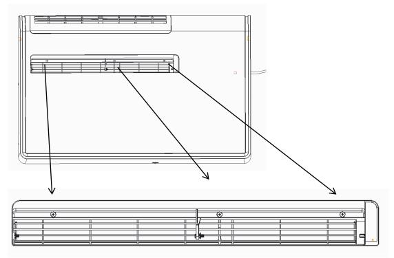
2. remove the 2 screws fixed on the electronic control box cover, remove the electronic control box cover, and pull out the connected terminal for subsequent disassembly and maintenance. .
