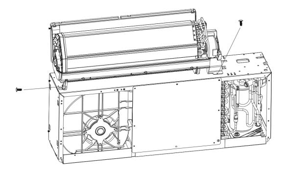
4. lift the evaporator assembly, tilt the inner machine base assembly out.
