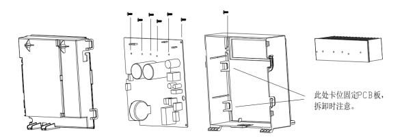
3. remove the 2 screws on the fixed heat dissipation fan bracket and remove the heat dissipation fan.
