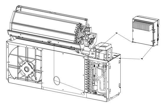
2. remove the screws fixing the main control PCB and remove the main control PCB. Remove the screws that fix the PCB radiator and the electronic control box and remove the PCB radiator.
