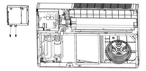
3. slightly lift the base with the hand, pull the front shell out, the left and right sides of the front shell and the machine left and right sides of the sheet metal joint clip to ensure that has been detached, the front shell bottom and the machine inside the base joint clip to ensure that has been detached, horizontal move out of the front shell, when moving out pay attention to loosen the connection line.
